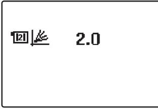
Set the heating curve steepness for the second heating circuit.
