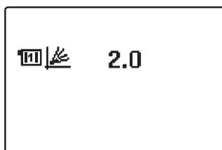
Set the heating curve steepness for the first heating circuit. Change the value with buttons ◀ and ▶. Confirm the selected value by pressing **OK**.
