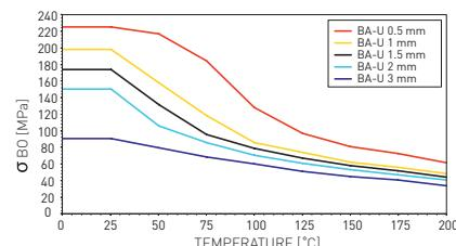
$\sigma_{Bo}$  diagrams represent  $\sigma_{Bo}$  values for different gasket material thicknesses. These values indicate the maximum in-service compressive pressures which can be applied on the gasket area involved without destroying or damaging the gasket material.
