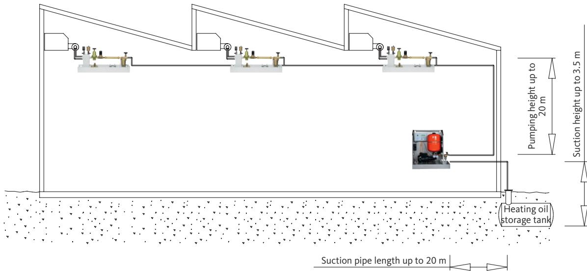
If pressure storage units are applied in systems with a very high degree of protection against failure required (e.g. in hospitals, production facilities, etc.), it is recommended to install a second unit to ensure a high system reliability.
