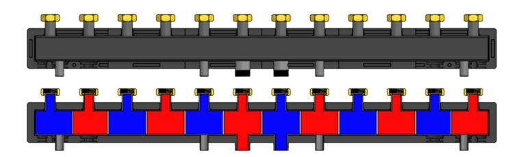
A DISTRIBUTOR IS DESIGNEG FOR CENTRAL HEATING INSTALLATION UP TO 120 KW WITH A POSSIBILITY OF CONNECTING 5 PUMP GROUPS. IT IS MADE OF STEEL, CLOSED IN A FOAMED POLYPROPYLENE INSULATION IN ORDER TO REDUCE HEAT LOSSES. IT IS USED TO FACILITATE ASSEMBLY OF MIXING AND PUMPING GROUPS. DISTRIBUTORS ALLOW TO USE A MUCH SMALLER NUMBER OF INSTALLATION DEVICES, WHICH SAVES SPACE, TIME AND REDUCE INSTALLATION COSTS. A SET INCLUDES HANDLES, SCREWS, EXPANSION BOLTS AND WASHERS FOR MOUNTING ON THE WALL.
