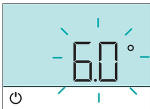
The temperature for frost protection can be set when the controller is switched off.
