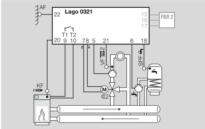
The heating controller controls the boiler, the mixer and the storage charging pump.
