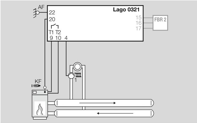
The heating controller controls the boiler and the pump for the direct heating circuit.
