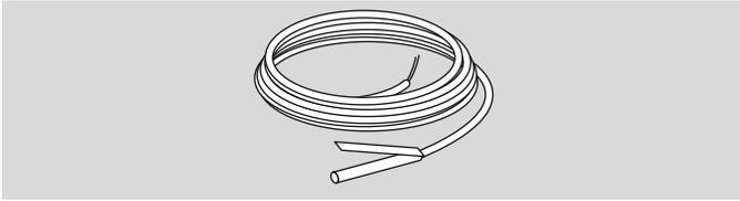
For measuring the flow or multifunction temperature. Installation for heating system control as close as possible behind the boiler on the heater flow pipe, for mixer operation approx. 0.5 m behind the heating circuit pump instead of a boiler sensor KF.
