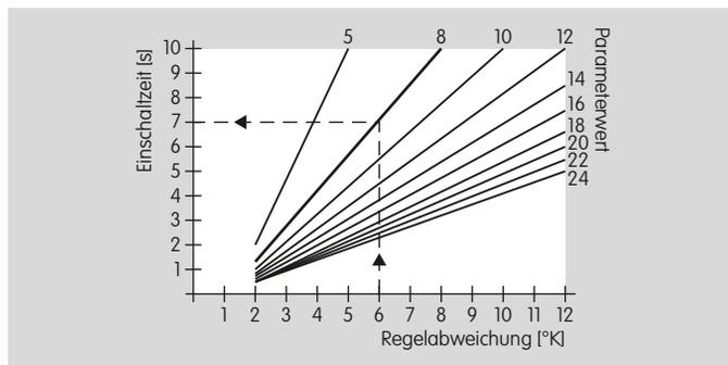
In the case of a controller deviation of 6 K, the mixer is actuated for 7 s and remains switched off for 3 s.
