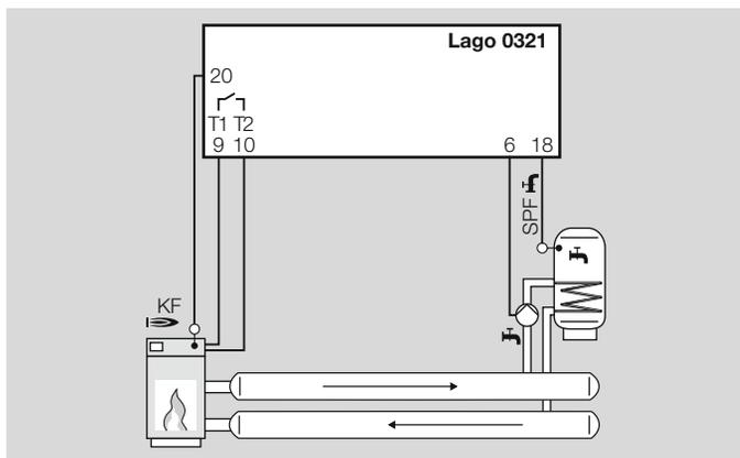
The heating controller controls the boiler and the storage charging pump.
