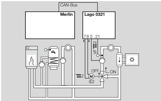
The mixer in the heating circuit functions as a valve. The mixer opens (ON). The heating circuit pump is switched on.
