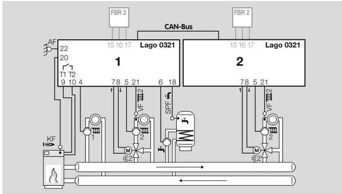
Heating controller 1 controls the boiler, the direct heating circuit, the mixed heating circuit and the storage charging pump. Heating controller 2 controls the extended mixed heating circuit. The heating controllers are linked via the CAN bus interfaces.
