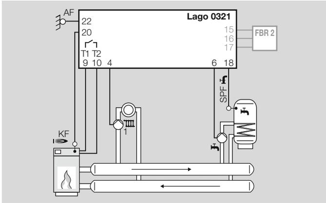
The heating controller controls the boiler, the direct heating circuit and the storage charging pump.
