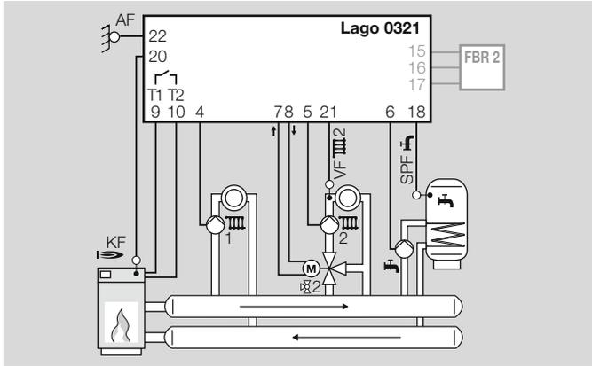
The heating controller controls the boiler, the mixer, the pump for the direct heating circuit (1<sup>st</sup> heating circuit) and the mixed heating circuit (2<sup>nd</sup> heating circuit), and the storage charging pump.
