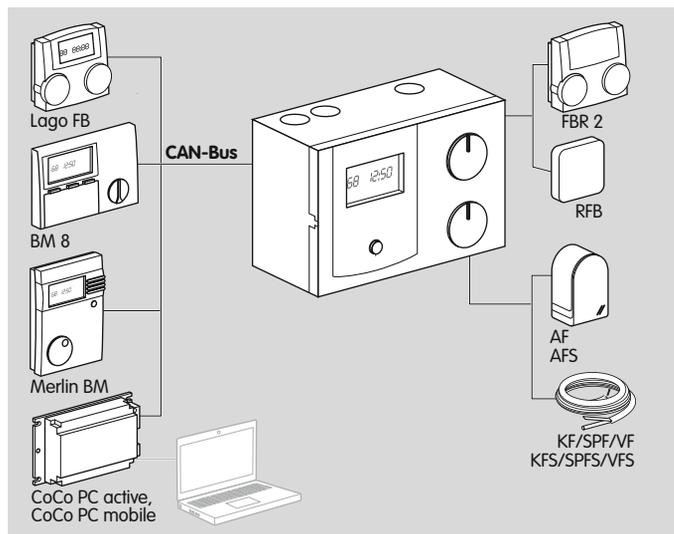
The Lago 0321 heating controller can control one direct heating circuit and one mixer circuit with a 3-way mixer at the same time. The connection possibility for the direct heating circuit can be used alternatively for a multifunction relay, e.g. for connection of a circulation pump, return flow booster or header pump.
