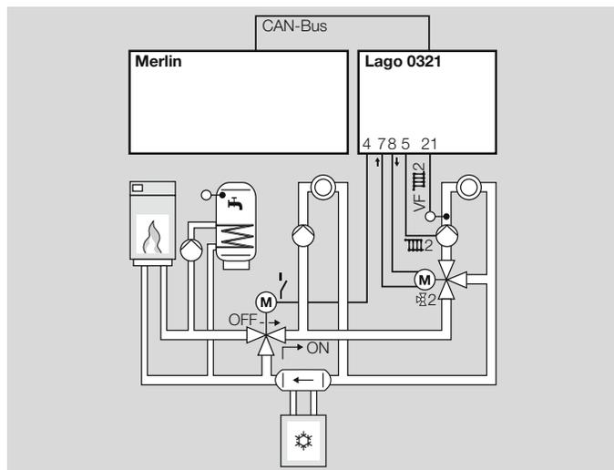
The central controller (e.g. Merlin) activates the “Cooling” operating mode via the CAN bus and controls the heat source, the refrigerating machine, the hot water preparation and the direct heating circuit. The Lago 0321 heating controller controls the bypass valve and the mixed heating circuit.
