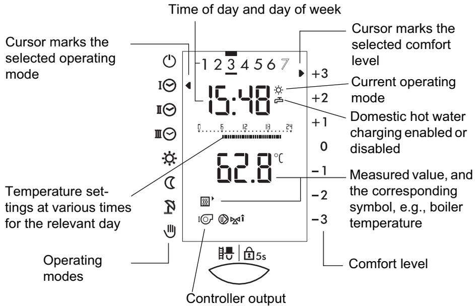
The diagram shows a display, with all the display symbols used for control.
