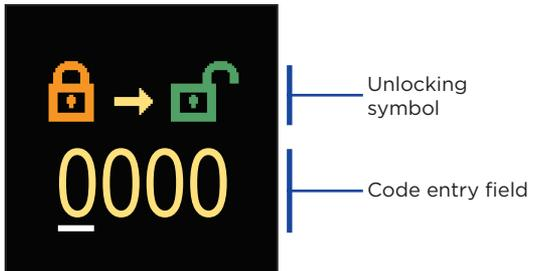
With the buttons ⊖ and ⊕ you change the value and with the button ⊙ you move on to the next position and confirm the unlocking.
