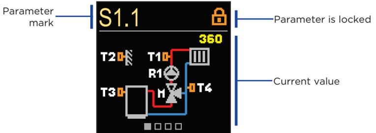
With the ⊖ and ⊕ buttons navigate through the parameters in the selected group. The parameter you want to change is selected by pressing the ⊙ button.
