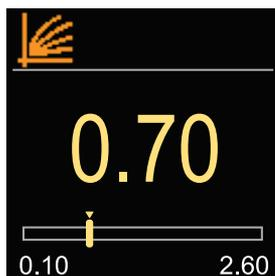
You can set the heating curve steepness. The steepness can be set with the buttons  $\ominus$  and  $\oplus$ .
