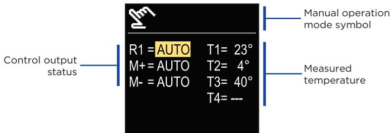
With the buttons  $\ominus$  and  $\oplus$  you can move between the individual outputs R1, M + or M-, and with the button  $\odot$  you can select the AUTO, OFF or ON status. Exit the setting by pressing  $\odot$ .
