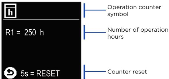
By pressing the button
