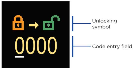
With the buttons  $\ominus$  and  $\oplus$  you can change the value and with the button  $\odot$  you can move on to the next position and confirm the unlocking. Exit the screen with the button  $\odot$ .
