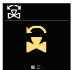
You can select the opening direction of the mixing valve. Use the buttons  $\bigcirc$  and  $\bigcirc$  to navigate between direc-
