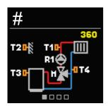
You can select the hydraulic scheme for the controller operation. Use the buttons  $\bigcirc$  and  $\bigcirc$  to navigate between schemes.
