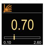
You can set the heating curve steepness. The steepness can be set with the buttons  $\bigcirc$  and  $\bigcirc$ . Confirm the set steepness with the button (•).
