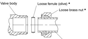
Pipe is slip fit into valve body
