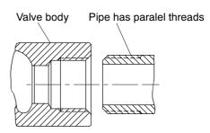
Fig. 16. 1/2" BSPP internal (Rp 1/2")
