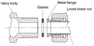
Pipe is soldered or threaded into metal flange (solder joint shown)
