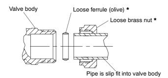
Using ferrule and nut for sealing 28 mm outerdiameter pipe. \* Compression nut and olive are supplied with the valve body.
