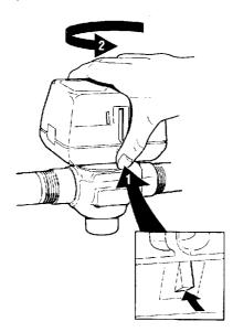
Fig. 11. Latch mechanism
