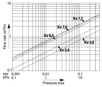
Fig. 8. Valve pressure loss characteristic for 3-way valves
