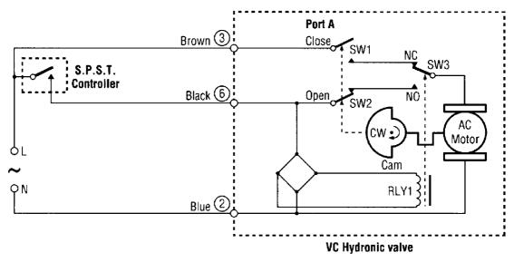
Fig. 4. Logic sequence diagram with 2 wire + common actuator for SPST controller
