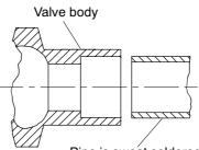
Pipe is sweat soldered into valve body
