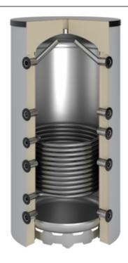
This buffer storage tank fulfills the highest demands on heat storage, particularly where heat generators are used which achieve their optimal efficiency only under full load (e.g. many solid fuel boilers). During the operation of the heat generator, more heat is produced than the consumers can take. The excess heat heats the water of the buffer tank and is therefore stored. During later stand-still periods this heat can be retrieved, as needed.
