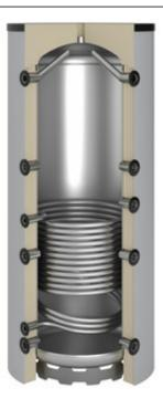
This buffer storage tank fulfills the highest demands on heat storage, particularly where heat generators are used which achieve their optimal efficiency only under full load (e.g. many solid fuel boilers). During the operation of the heat generator, more heat is produced than the consumers can take. The excess heat heats the water of the buffer tank and is therefore stored. During later stand-still periods this heat can be retrieved, as needed.
