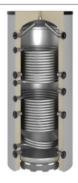
This buffer storage tank fulfills the highest demands on heat storage, particularly where heat generators are used which achieve their optimal efficiency only under full load (e.g. many solid fuel boilers). During the operation of the heat generator, more heat is produced than the consumers can take. The excess heat heats the water of the buffer tank and is therefore stored. During later stand-still periods this heat can be retrieved, as needed.
