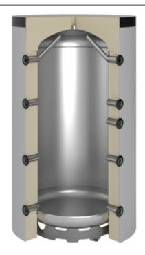
This buffer storage tank fulfills the highest demands on heat storage. Due to its highly efficient insulation, the heat-retaining loss is significantly reduced compared to common storage tanks. The purpose of the buffer storage tank is to balance the difference between generated heat and consumed heat. So the heat generators can be operated more independently from the consumption.
