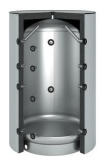
This OEG buffer storage tank fulfills the highest demands on heat storage. Due to its highly efficient insulation, the heat-retaining loss is significantly reduced compared to common storage tanks. The purpose of the buffer storage tank is to balance the difference between generated heat and consumed heat. So the heat generators can be operated more independently from the consumption.
