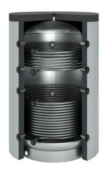
This OEG buffer storage tank fulfills the highest demands on heat storage, particularly where heat generators are used which achieve their optimal efficiency only under full load (e.g. many solid fuel boilers). During the operation of the heat generator, more heat is produced than the consumers can take. The excess heat heats the water of the buffer tank and is therefore stored. During later stand-still periods this heat can be retrieved, as needed.
