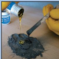
2. Mix the two components carefully. For ratio see text at top right.
