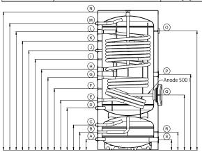
When using the storage tank as cold storage tank, all connections, also the ones currently not used, must be insulated impermeably.\*
