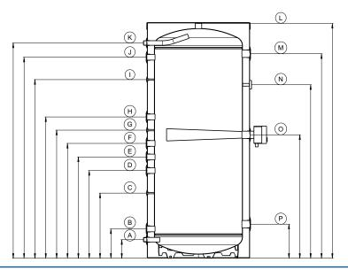
When using the storage tank as cold storage tank, all connections, also the ones currently not used, must be insulated impermeably.\*
