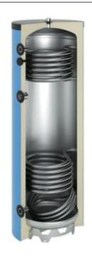
This OEG buffer storage tank fulfills the highest demands on heat storage, particularly where heat generators are used which achieve their optimal efficiency only under full load (e.g.: many solid fuel boilers). During the operation of the heat generator, more heat is generated than is retrieved by the consumers. The excess heat then heats up the water of the buffer tank and is stored there.
