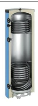
This OEG buffer storage tank fulfills the highest demands on heat storage, particularly where heat generators are used which achieve their optimal efficiency only under full load (e.g.: many solid fuel boilers). During the operation of the heat generator, more heat is generated than is retrieved by the consumers. The excess heat then heats up the water of the buffer tank and is stored there.
