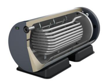
The structure of these storage tanks is fundamentally different from usual large-volume domestic water tanks. A built-in corrugated stainless steel pipe separates the drinking water from the heating water and serves as a powerful heat exchanger at the same time. Thus, the advantages of a buffer tank are combined with those of a flow heater.
