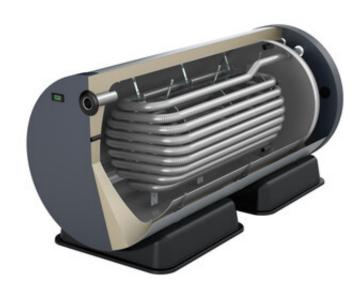
The structure of these storage tanks is fundamentally different from usual large-volume domestic hot water tanks. A built-in corrugated stainless steel pipe separates the drinking water from the heating water and serves as a powerful heat exchanger at the same time. Thus, the advantages of a buffer tank are combined with those of a flow heater.
