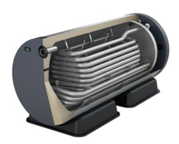
The structure of these storage tanks is fundamentally different from usual large-volume domestic water tanks. A built-in corrugated stainless steel pipe separates the drinking water from the heating water and serves as a powerful heat exchanger at the same time. Thus, the advantages of a buffer tank are combined with those of a flow heater.
