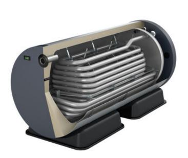
The structure of these storage tanks is fundamentally different from usual large-volume domestic water tanks. A built-in corrugated stainless steel pipe separates the drinking water from the heating water and serves as a powerful heat exchanger at the same time. Thus, the advantages of a buffer tank are combined with those of a flow heater.
