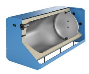
Horizontal buffer storage tank as built-under storage tank for oiland gas-condensing boilers of almost any manufacturer. The stable construction allows loads of up to 500 kg. The unrivalled OEG vacuum insulation of the storage tanks has significantly lower heat losses than the insulation of common storage tanks available on the market.
