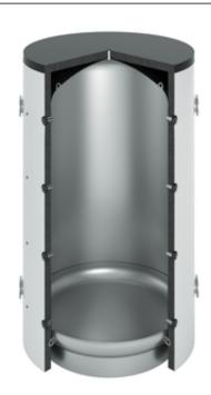
This buffer storage tank fulfills the highest demands on heat storage. Due to its highly efficient insulation, the heat-retaining loss is significantly reduced compared to common storage tanks. The purpose of the buffer storage tank is to balance the difference between generated heat and consumed heat. So the heat generators can be operated more independently from the consumption.
