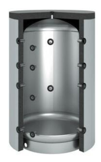
This OEG buffer storage tank fulfills the highest demands on heat storage, particularly where heat generators are used which achieve their optimal efficiency only under full load (e.g. many solid fuel boilers). During the operation of the heat generator, more heat is produced than the consumers can take. The excess heat heats the water of the buffer tank and is therefore stored. During later stand-still periods this heat can be retrieved, as needed.
