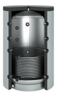
This buffer storage tank fulfills the highest demands on heat storage, particularly where heat generators are used which achieve their optimal efficiency only under full load (e.g. many solid fuel boilers). During the operation of the heat generator, more heat is produced than the consumers can take. The excess heat heats the water of the buffer tank and is therefore stored. During later stand-still periods this heat can be retrieved, as needed.
