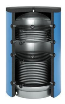
This buffer storage tank fulfills the highest demands on heat storage, particularly where heat generators are used which achieve their optimal efficiency only under full load (e.g. many solid fuel boilers). During the operation of the heat generator, more heat is produced than the consumers can take. The excess heat heats the water of the buffer tank and is therefore stored. During later stand-still periods this heat can be retrieved, as needed.
