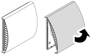
4. Fix the back wall of the ventilation hood on the wall using the supplied screws 4x40.
