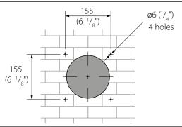
3. Insert the supplied expansion anchors 6x40 into the holes. Disassemble the outer ventilation hood to enable access to the fastening holes.
