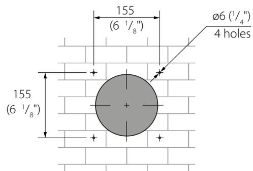
3. Insert the supplied expansion anchors 6x40 into the holes.
