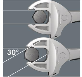
Thanks to the corner-width rectangular prisms, a back-pivoting angle of only 30° can be realized.
