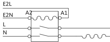
E2: Electrical booster heater for heating water
