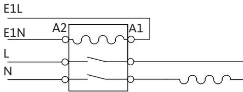
E1: Electrical booster heater for hot water
