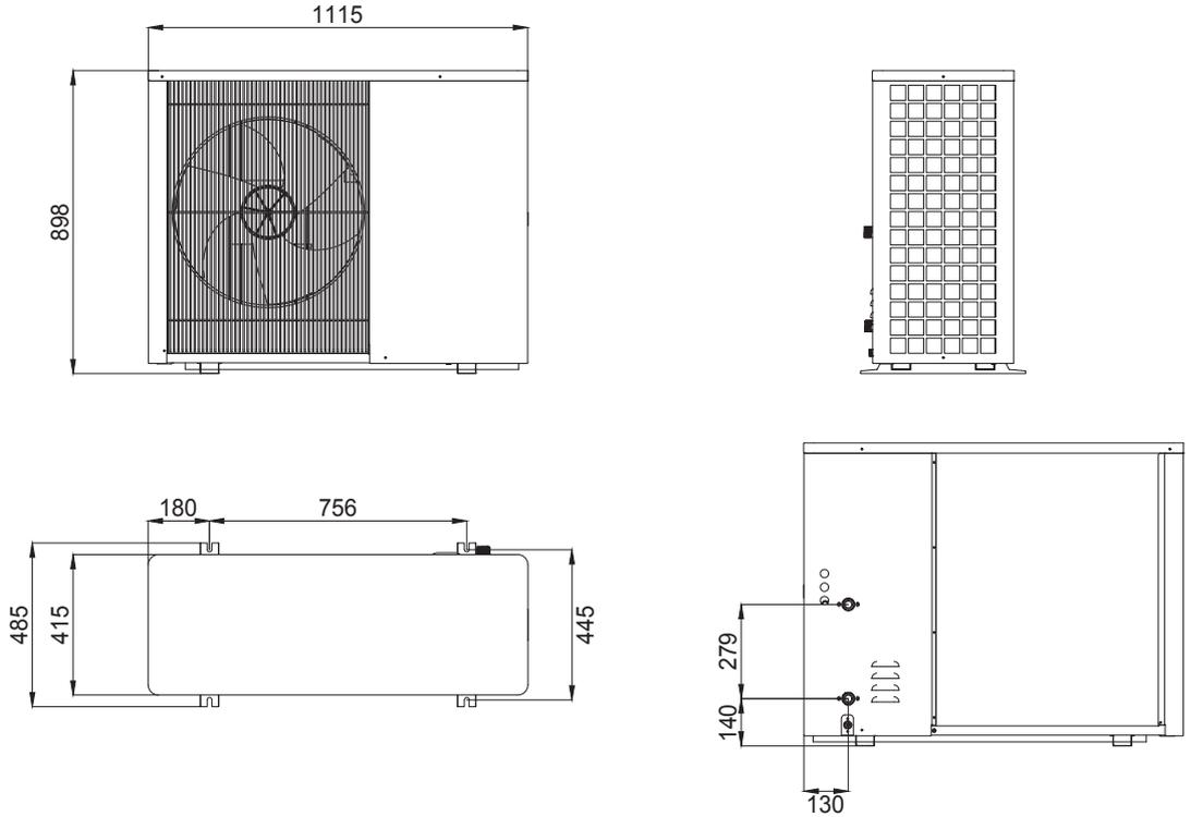
650 001 332 – Air/water heat pump 12 kW R290 Inverter 400 V
