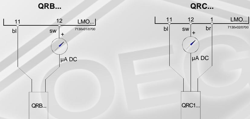
As an alternative to the detector current measurement, the diagnostic tool OCI400 / ACS400 can be used. In that case, connection of the DC microammeter is not required.
