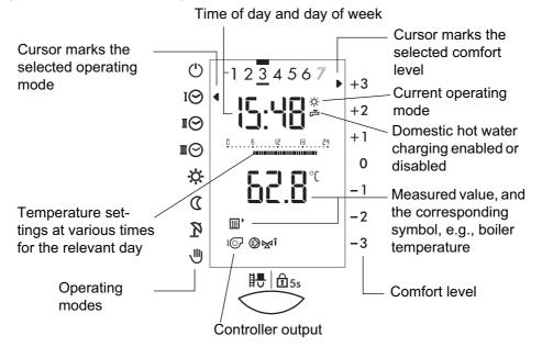
The diagram shows a display, with all the display symbols used for control. (cover open, User Level 2.).
