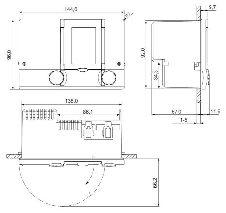
The installation space amounts to 92 (0/+1) x 138 (0/+1) mm in accordance with DIN 43700. Instrument panel strengthens <5 mm
