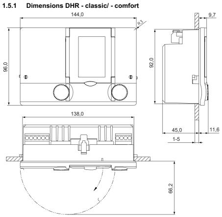
The installation space amounts to 92 (0/+1) x 138 (0/+1) mm in accordance with DIN 43700. Instrument panel strengthens <5 mm
