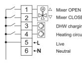
(M1) Mixer CLOSE DHW charging pumpe (L) Heating circuit pump (U1) Live Neutral
