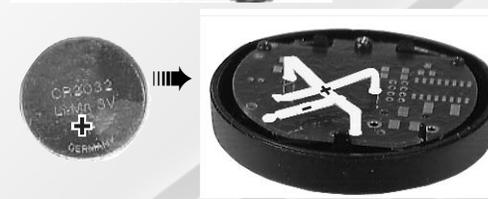
The battery has to be changed if the symbol appears in the display during the measurement. Open the housing using a screwdriver. Remove the used button cell. Put in new button cell - **Observe polarisation!**
