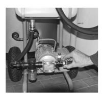
Connect pressure hose to pump outlet
