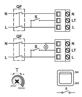
S - external switch QF - Linematic switch
