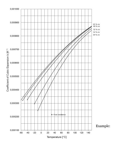
By how much does  $V_0$  = 100 L of a 35 % v/v Antifrogen® N/ water mixture expand on heating from  $t_0$  = -10 °C to  $t_1$  =80 °C?
