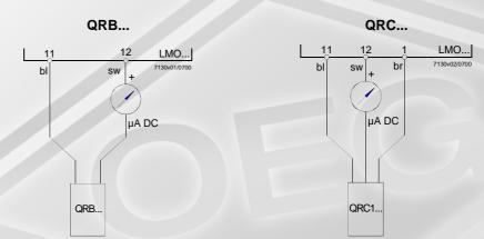
As an alternative to the detector current measurement, the diagnostic tool OCI400 / ACS400 can be used. In that case, connection of the DC microammeter is not required.
