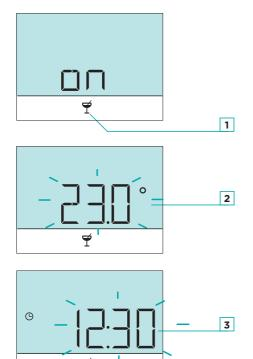
By pressing the  $\equiv 3$  button, you select the requested function  $\stackrel{\checkmark}{T}$  and confirm it with the  $\checkmark$  button.
