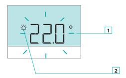
By pressing the + or - button, you activate the requested temperature setting. The current active temperature (day or night) starts flashing.
