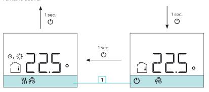
\* Heating or cooling of rooms and heating of domestic hot water according to the time programme is active. \* Domestic hot water heating according to the time programme and frost or overheating protection is active.
