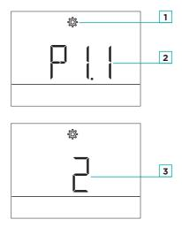
When entering submenu P1, P2, or S1, you can browse through the parameters with lacktriangle and lacktriangle .
