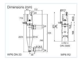
According to EN 12828, sealed heating systems with capacities of more than 300 kW must be equipped with a TÜV-tested boiler water low level alarm.
