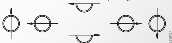
The layout of piping must ensure that the meter is at all times filled with liquid and that no inclusions of air or gas may occur.
