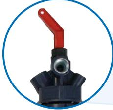
Quick-action shut-off valve with lever for fast shutting off of the oil supply. Remote operation from outside of the tank room possible with pull cord.
