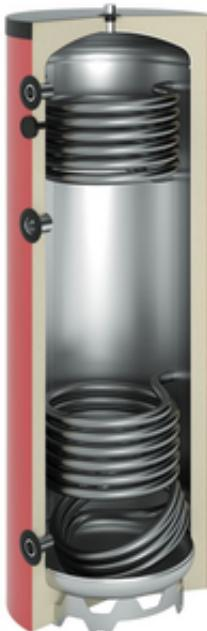
This OEG buffer storage tank fulfills the highest demands on heat storage, particularly where heat generators are used which achieve their optimal efficiency only under full load (e.g.: many solid fuel boilers). During the operation of the heat generator, more heat is generated than is retrieved by the consumers. The excess heat then heats up the water of the buffer tank and is stored there.
