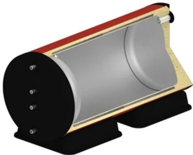
Horizontal buffer storage tank for positioning below sloping roofs, staircases and where the ceiling height is not sufficient for standard vertical storage tanks. The unrivalled OEG vacuum insulation of the tanks has significantly lower heat losses than the insulation of common storage tanks available on the market.
