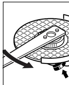
A properly attached, undamaged quick-clamping nut can be loosened by hand when turning the knurled ring in anticlockwise direction.
