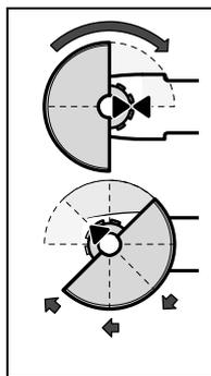
Place the protection guard **11** onto the spindle collar as shown in the illustration. The triangle marks on the protection guard must correspond with the respective marks on the gear case.
