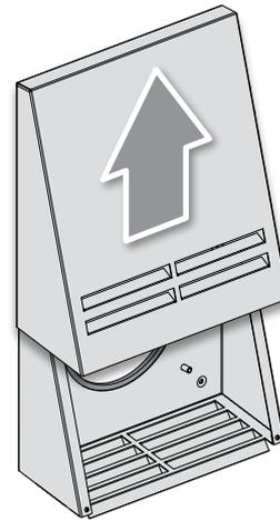
4. Fix the back wall of the ventilation hood on the wall using the supplied screws 4x40.
