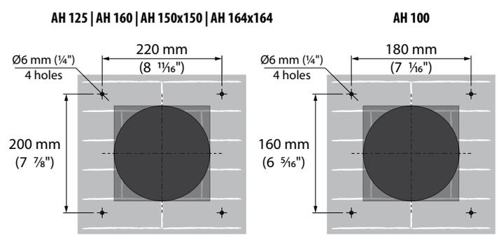
3. Insert the supplied expansion anchors 6x40 into the holes. Disassemble the outer ventilation hood to ensure access to the fastening holes. Remove the ventilation hood front part.
