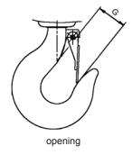
As hook dimensions can change from one to another due to forging toleraces, the user should measure the exact dimension "G" at the supplied hoist and logg it to this table.
